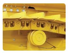
Individual links can be replaced with common track tools
