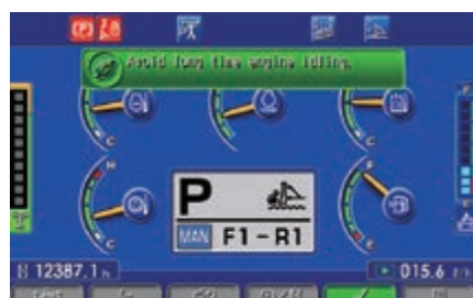
Eco-gauge, Eco guidance and fuel consumption gauge
