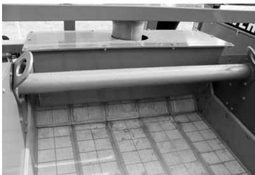
Modular screen decks and side protection liners
