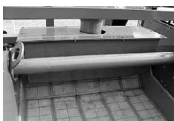
Full width underflow distribution box giving and even flow to the screen
