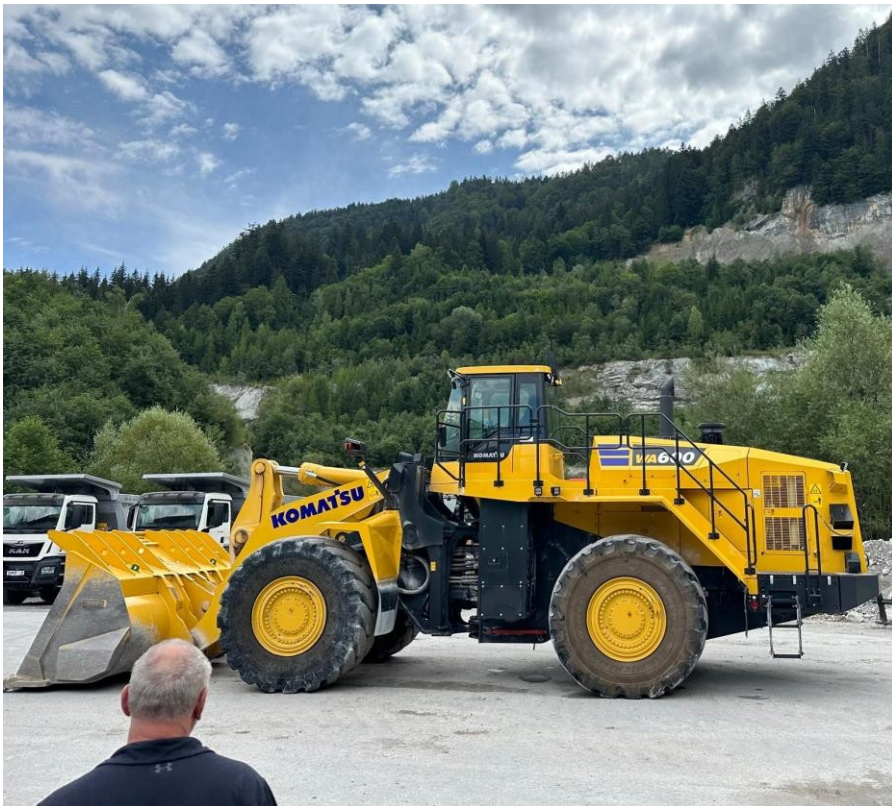
The WA600-8 wheel loader from Komatsu provides unbeatable productivity and fuel efficiency with its optional torque converter lock-up.
